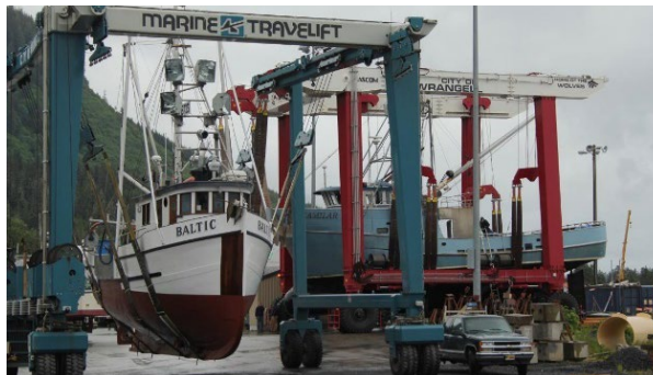
Wrangell's 300-ton and 150-ton boat lifts in operation
