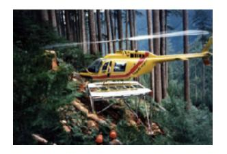
See photos for examples of the portable/removable helipads. They can be constructed on site, or flown in, and easily adapt to undulating or sloping land.
