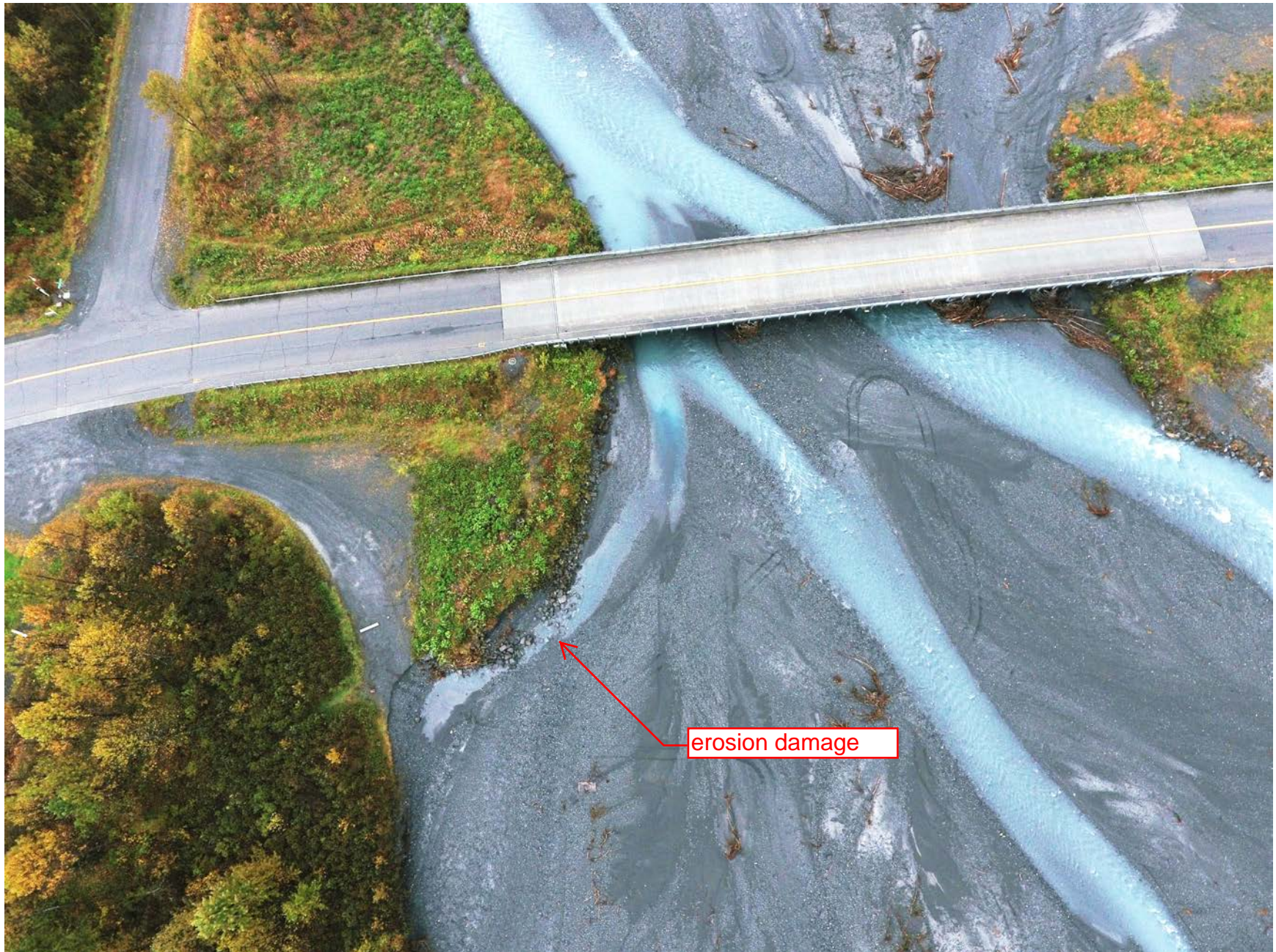
Birds eye view of the damaged area upstream of the bridge on the Blueberry Hill road side.
