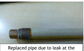
Replaced pipe due to leak at the transition on LH end of pipe. No pipe support provided.
