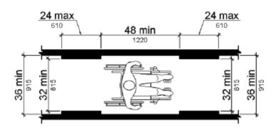
Figure 403.5.1 Clear Width of an Accessible Route
