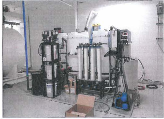
Assembling Oil Trap bilge treatment equipment
