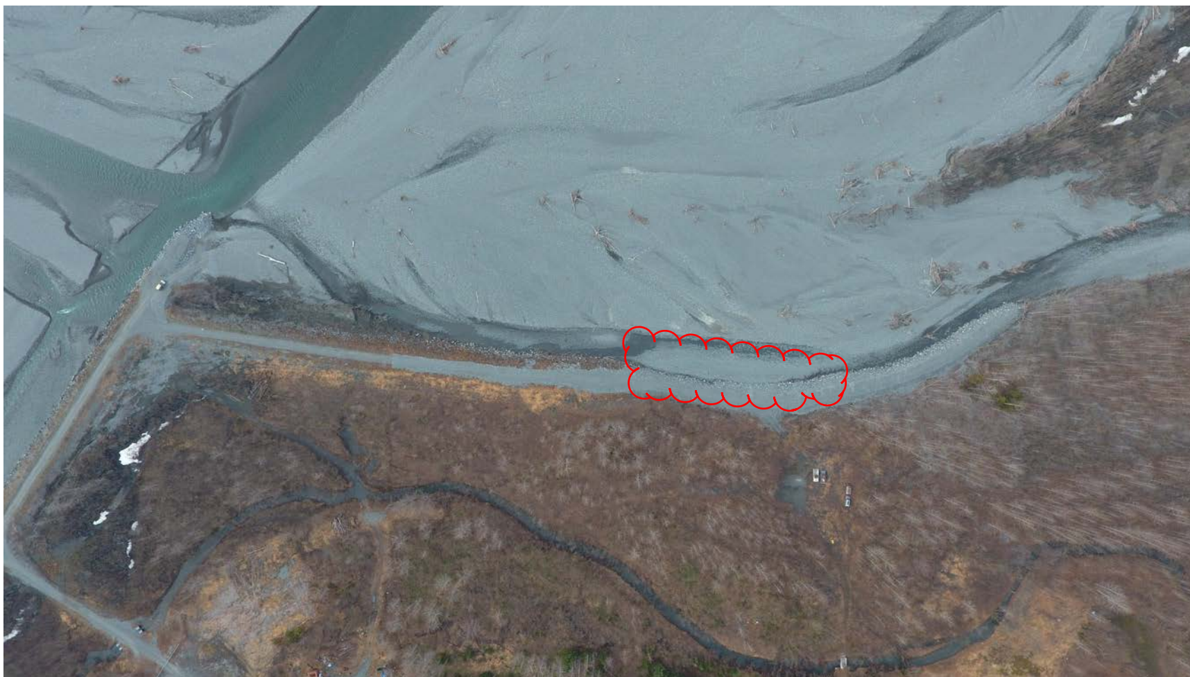
Overhead view of groin #4 and the eroded area that will be reinforced with riprap.
