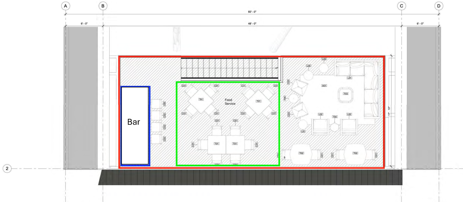
1 FLOOR PLAN - MEZZANINE FF&E ID501 3/8" = 1'-0"
